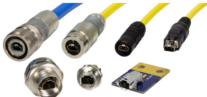
SPE connector variants according to IEC 63171-6: as IP65/67 as well as IP20 versions (upper row from left to right: M12 PushPull, M8 PushPull, M8 SnapIn and IP20 connectors / upper row from left to right: M12 socket with screw and PushPull interlocks, M8 socket with SnapIn and PushPull interlocks, angled IP20 PCB socket)
