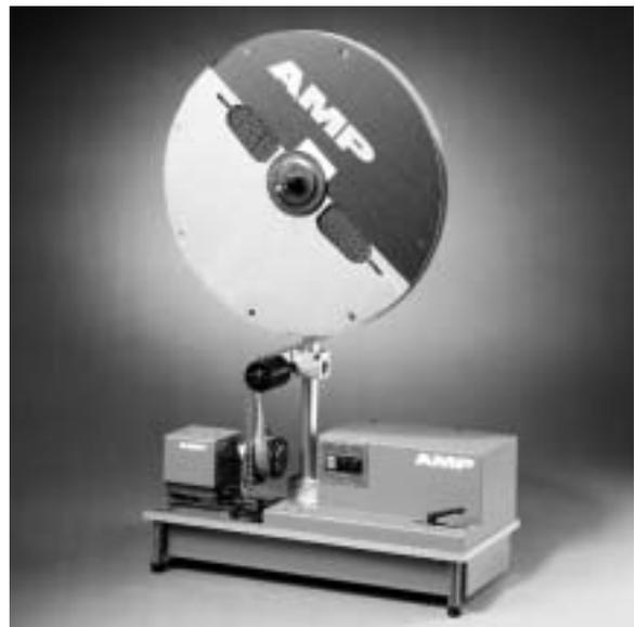
**Connector dispenser PN 677463-1.** The dispenser accepts the Micro-MaTch standard reels (2500 pcs/reel). It automatically removes the pre-set connector quantity from the reel and drops it in a separate box. Quantity can easily be programmed by the user.
