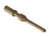
Series 927-072 contacts for size #16s through size #0 wire. Copper alloy with silver or gold plating, Terminate to wire with standard crimp tools. Contacts are front-release. Use in series 927-072 connectors.
