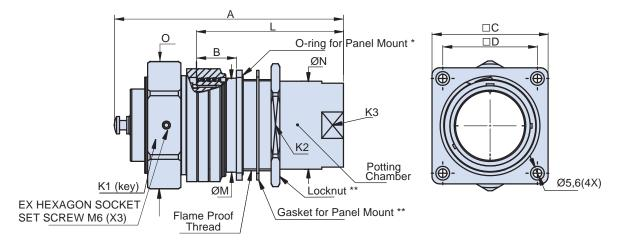
(\*) For Mounting on Ex d enclosure: use only O-ring for Panel Mount. (\*\*)For Mounting on Ex e enclosure: use only Gesket for Panel Mount and Locknut.
