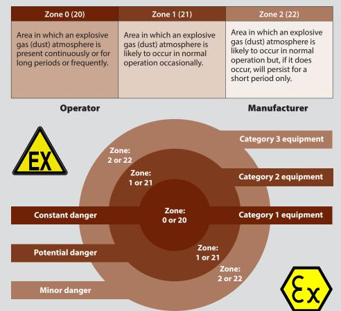
Explosive area zone classifications are used by the operator to distinguish between explosive areas and their relative levels of risk. Operators use the triangular EX mark to indicate compliance with IECEX/ATEx requirements. Manufacturers however use different classifications to describe where their products may be used. The two systems generally conform in meaning but the words and symbols change.
