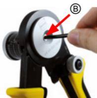
2. Insert a properly stripped wire into the crimp contact ②.
