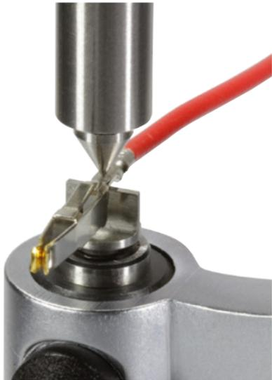
Figure V-10: Detail view of crimp contact
