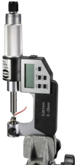
Figure V-9: Micrometer screw
