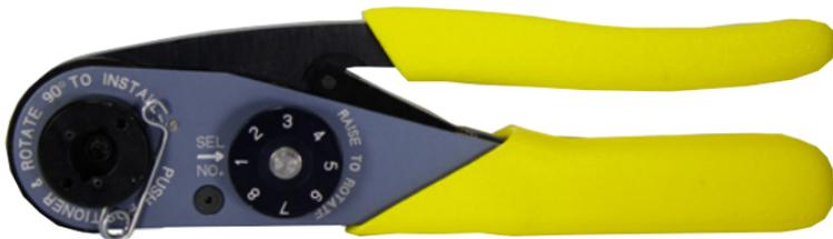
Figure V-14: Manual crimping tool 09 99 000 0501
