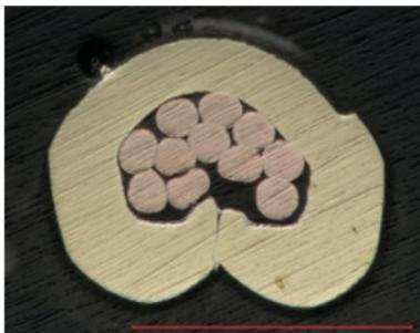
Figure V-7: Micro-section of a defective sample, wire cross-section too small
