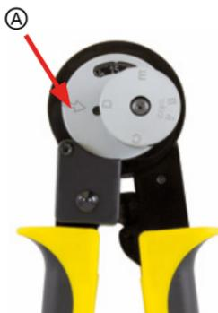
The arrow <sup>Ⓐ</sup> will indicate the selected marking. The locator will latch back into position when you release it.
