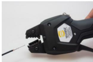
7. Remove the cable end with the crimped contact and carry out a visual inspection.
