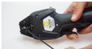
4. Fix the positioned contact and insert the stripped wire.
