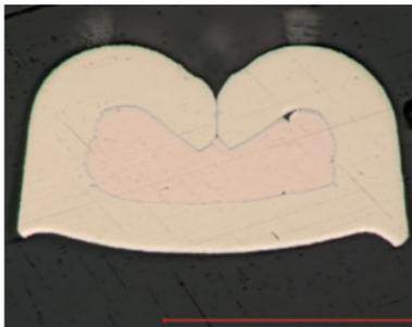
Figure V-5: Micro-section of a flawless sample
