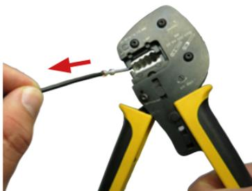
3. Upon release, the handles will open automatically and the crimped contact can be removed.
