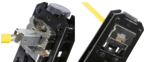
10. Add the lower shielding shell; snap it together with the upper shielding shell until it engages with an audible click.
