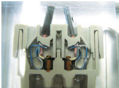
Figure VI-5: Termination with stripped stranded wire
