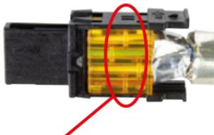
IDC – Position of the insulation displacement contact
