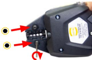
5. Use a 2.5 mm Allen key to tighten both fixing screws (⇒ red arrows). The recommended torque is 2.0 Nm.
