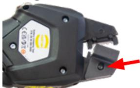
7. Insert the locator in the designated position and fix it with the supplied screw (⇒ red arrow).
