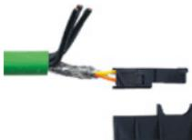
10. Put on the upper shielding shell and press it over the cable screen. Add the lower shielding shell; snap it together with the upper shield until it engages with an audible click.
