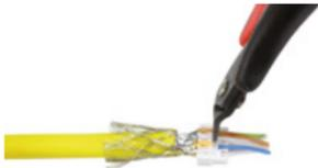
5. Press the wire manager and cable into the HARTING RJ Industrial® RJ45 module.
