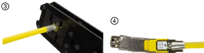
4. Insert the terminal module into the connector.
