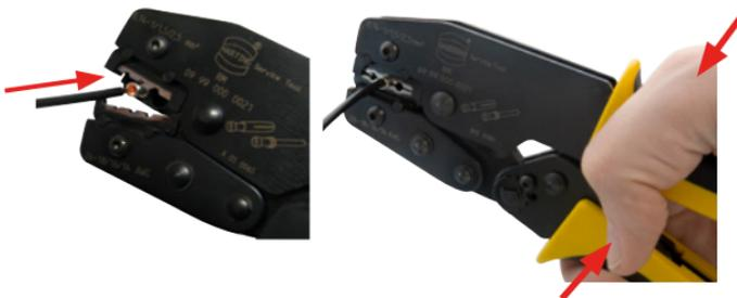
3. Remove the crimped contact.
