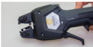
3. Lower the release lever so that the die opens and the contact can be re-adjusted if necessary.
