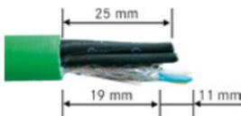
4. Prepare the wires for insertion into the splice element according to the colour coding.
