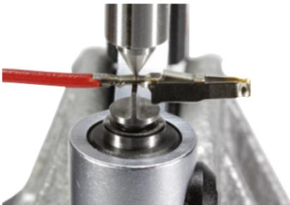
Figure V-11: Detail view of a crimp contact
