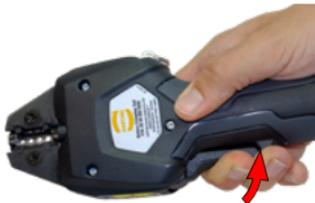
3. Pull up the release lever until the crimp die closes firmly and both parts of the crimping die hold position.
