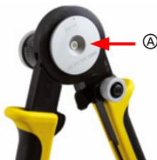
1. Insert the crimp contact into the tool opening ①. The locator ensures that the crimp contact is automatically positioned in the proper crimping position.
