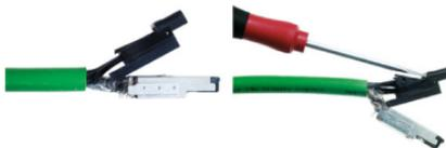
13. Metal housing: Push the housing over the assembled data module and insert. Secure the insert using the housing's locking screw. Tighten this screw using 0.5 Nm torque.
