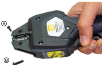
4. Keep the tool closed so that the upper and lower crimp die remain fixed in the correct position until you tighten the screws.
