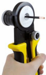
3. Press the crimping tool's handles together in order to crimp the contact. Press the handles closed until they automatically reopen (refer also to the chapter Ratchet lock, p. 79).
