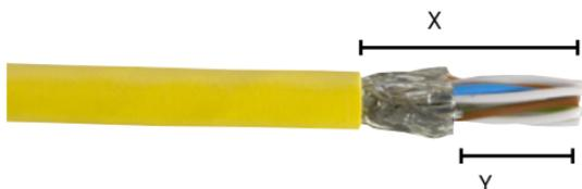
3. To guarantee simple assembly, check the stripping lengths from the following drawing at a 1:1 scale.
