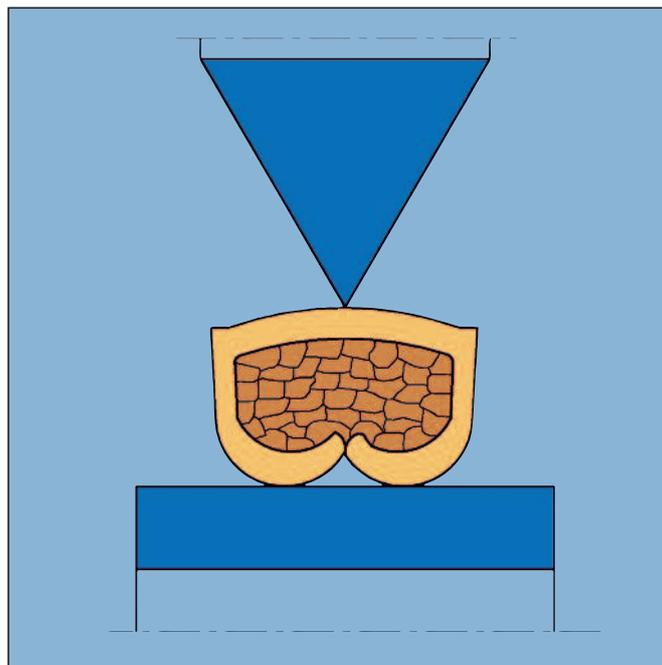
Due to the large degree of tolerance of the external diameter of the lead a crimping height is not specified.
