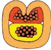
Insulation is pierced and could damage conductor
