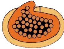
Insulation is over crimped
